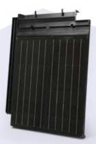
**CERASOLPAN** power: 175 Wp/m<sup>2</sup> weight: 18 kg/m<sup>2</sup> roof pitch starting at 18°
